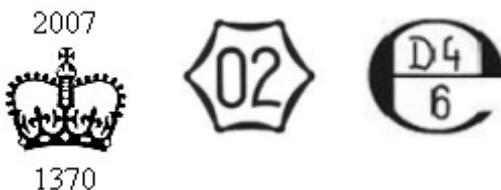
As with weighing equipment any weights that bear a six-pointed star stamp were found to be inaccurate when they were last inspected and would be illegal for use for legal weighing purposes.
