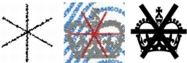
The six-pointed star stamp or sticker is applied to approved equipment that has been 'rejected' as it was found on inspection to be inaccurate or not in compliance with manufacturing requirements. It also indicates that the equipment has not since been adjusted or repaired.
